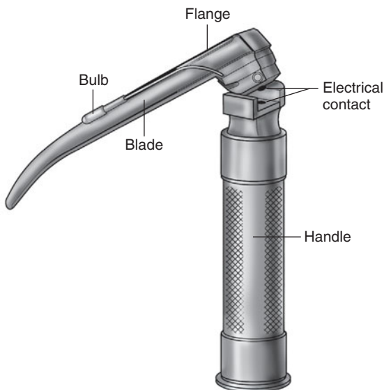
FIGURE 19-15 A rigid laryngoscope.
